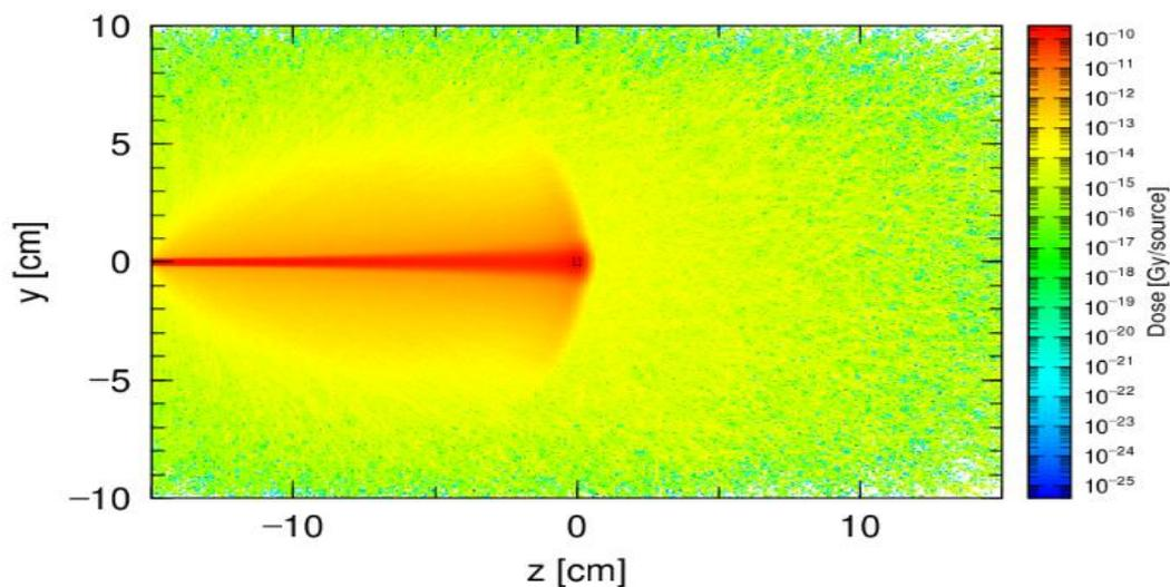
Fig. 4 2D view of dose profile for proton beam. Black box in the center is targeted volume.
