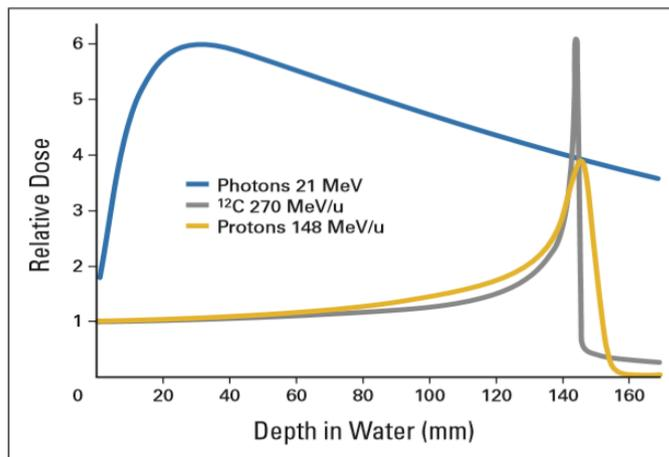
Fig. 1 Depth-dose profiles of photon, proton and carbon ion. Target material is water. Depth-dose curves of photon and proton are normalized so that they contribute same dose at 145mm. For same entrance dose as proton, carbon ion shows sharper Bragg peak. Figure from Schulz-Ertner and Tsujii [2].
