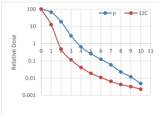
Fig. 6 Relative dose in targeted volume and boxes along vertical Y-axis. X-axis values on the graph represents box number in order. 0 is targeted volume. X-axis values 1-10 are boxes ordered from nearest to farthest distance from targeted volume.
