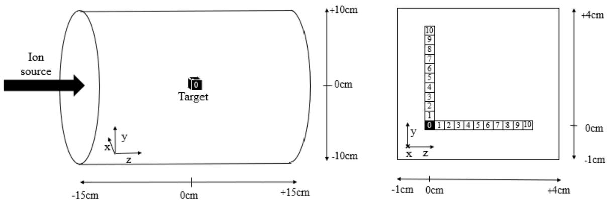
Fig. 3 (a) 3D view of constructed geometry and (b) Enlarged view of part of cylinder region on YZ plane. Box no.0 is targeted volume. Extra boxes are located along vertical Y-axis and along horizontal Z axis. All boxes are situated on the same YZ plane.
