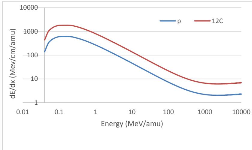
Fig. 2 Bethe equation solved for proton and carbon ion beam. Target material is water phantom. X-axis represents Energy per amu. Y-axis represents ionization energy loss divided by mass number. For ionization energy loss of carbon ion, Y-axis value must be multiplied with mass number of carbon ion, 12.
