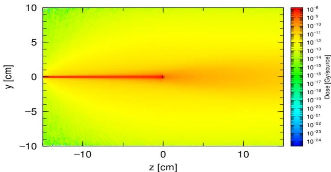
Fig. 5 2D view of dose profile for carbon beam. Black box in the center is targeted volume.
