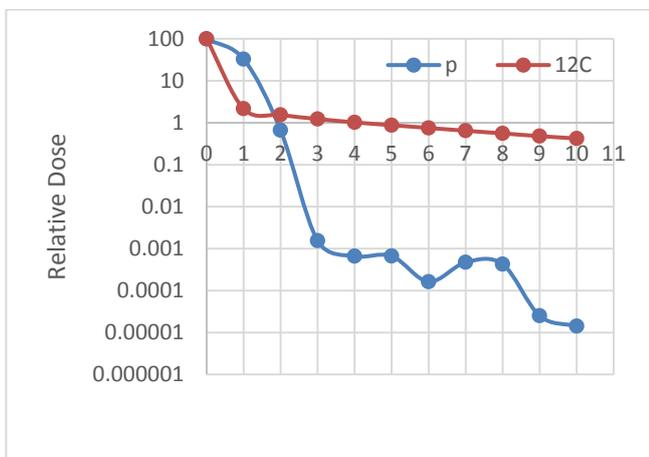
Fig. 7 Relative dose in targeted volume and boxes along horizontal Z-axis. X-axis values on the graph represents box number in order. 0 is targeted volume. X-values 1-10 are boxes ordered from nearest to farthest distance from targeted volume, similarly.
